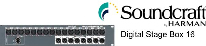
The Mini Stagebox 16 is a 2U chassis with 16 analog mic/line inputs and 8 line outputs for a 16 x 8 matrix. Mini Stagebox units interface with any of the Soundcraft Si Expression, Si Compact, Si Performer, Si Series and Vi Series consoles via an included MADI card fitted to the option card slot.
