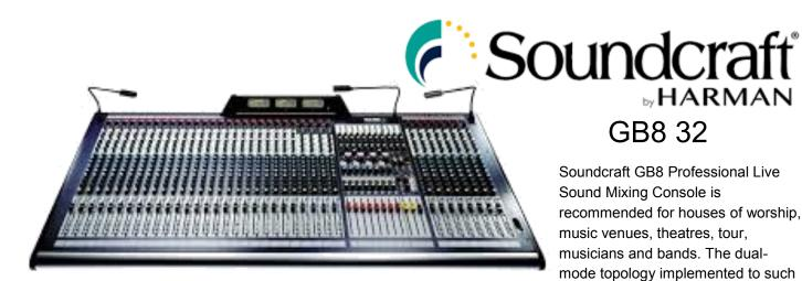
success on the MH3 and MH4 desks allows the GB8 to be used on FOH or monitor duties, with fader control of group or aux outputs.
