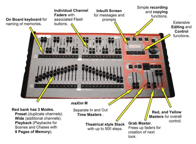
The **S** and **M** models are very similar, varying only in their number of faders and memories. At any point in this manual where the model affects the specification, the text will describe the *maXim* **S** followed by the *maXim* **M** in brackets.
