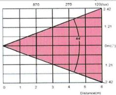
The Projector is best to be placed 5 meters from wall, and from this distance the light effect will cover an area of 4 m  $\times$  4 m.
